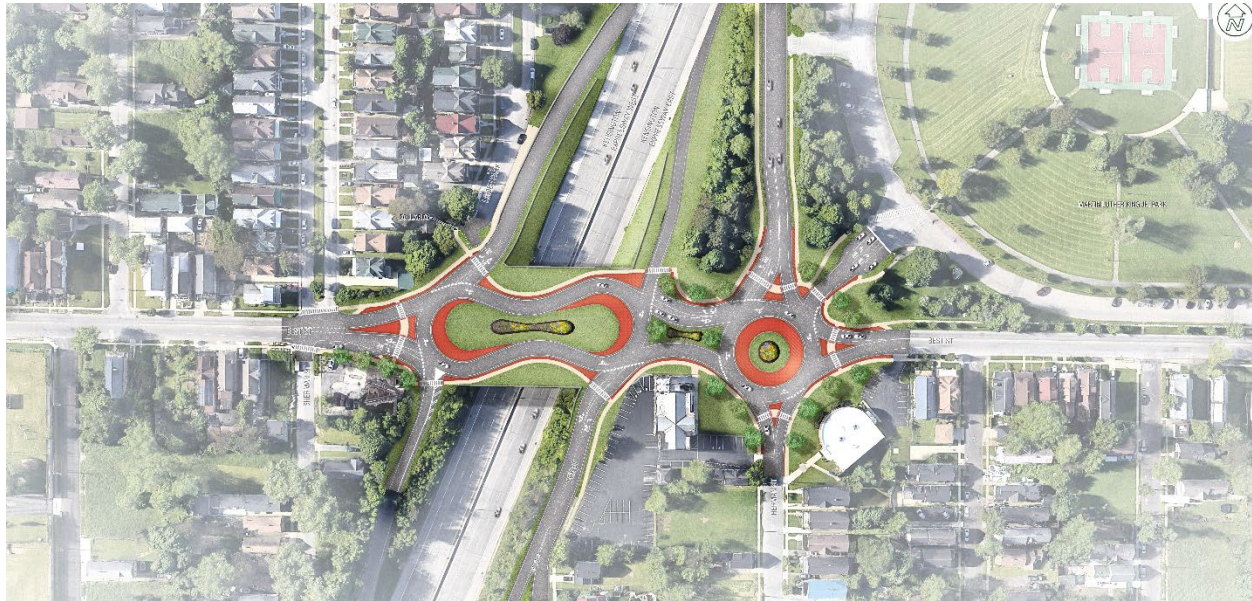
Figure 3: Plan of Best Street crossing and roundabout under the Build Alternative between Wohlrs Avenue and Rich Street.
